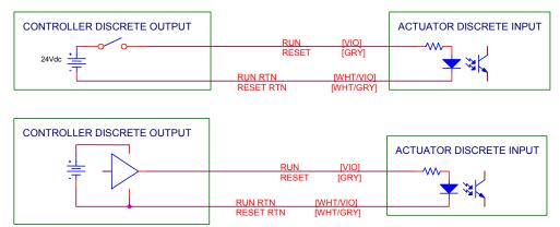
Figure 2-3: Typical Discrete Command Connection
